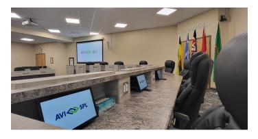
NEC projectors are mounted to the ceiling, projecting content on Da-Lite screens on either side of the space for official and in-room audience viewing. Wall-mounted 4K PTZ cameras and Voice Lift speakers capture city official and constituent interactions, supporting clear in-room communication.
